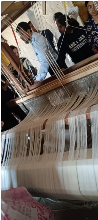
Fig 7, 8 & 9. Thread beam Preparation according to width & accurate thread count
