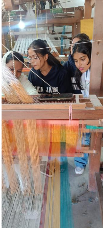
Fig 7, 8 & 9. Thread beam Preparation according to width & accurate thread count
