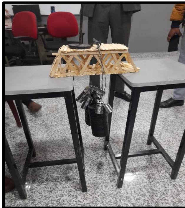
FIG 4: LOAD CAPACITY TEST OF THE MODEL
