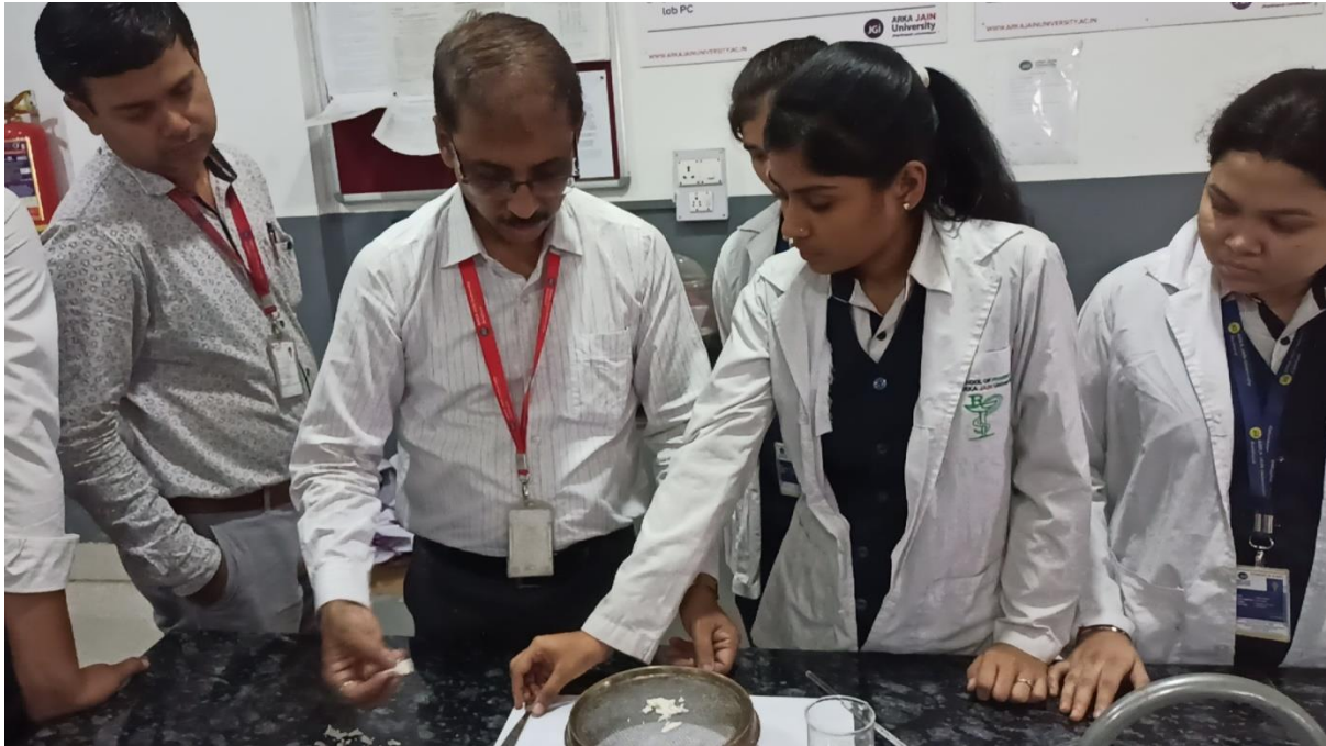
Passing the solidified mass to sieve number 10 to obtain the embedded matrix
