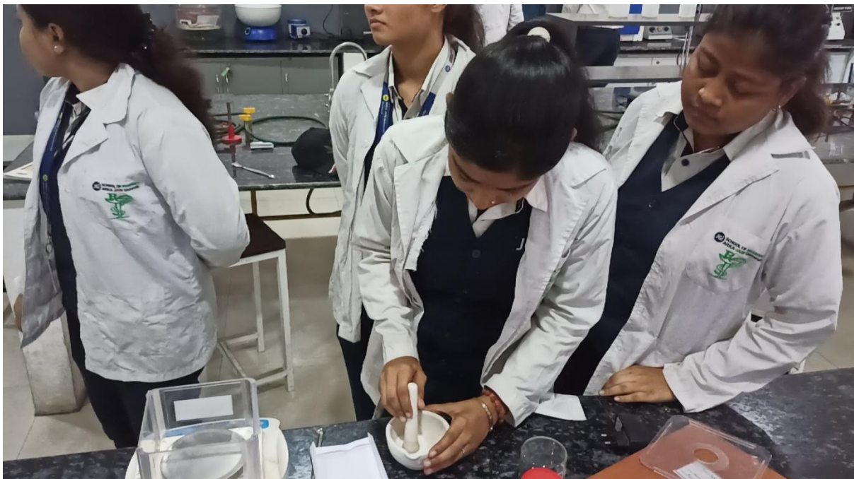
Further size reducing using mortar and pestle
