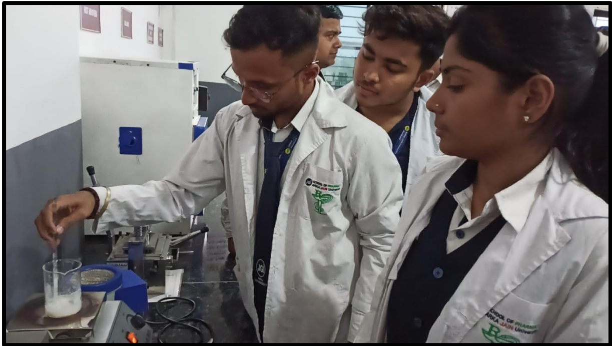
Figure 13: Dispersing aspirin to melted beeswax for embedding
