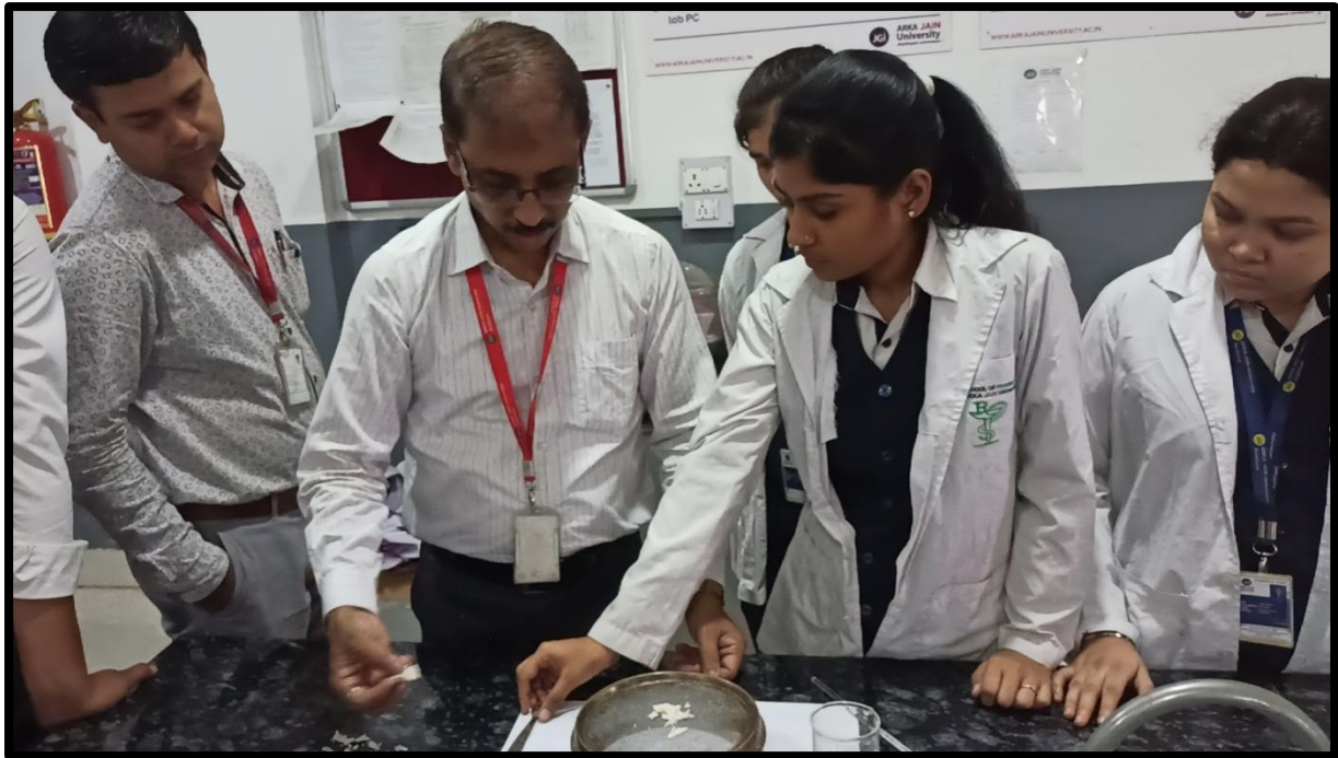
Figure 15: Passing the solidified mass to sieve number 10 to obtain the embedded matrix
