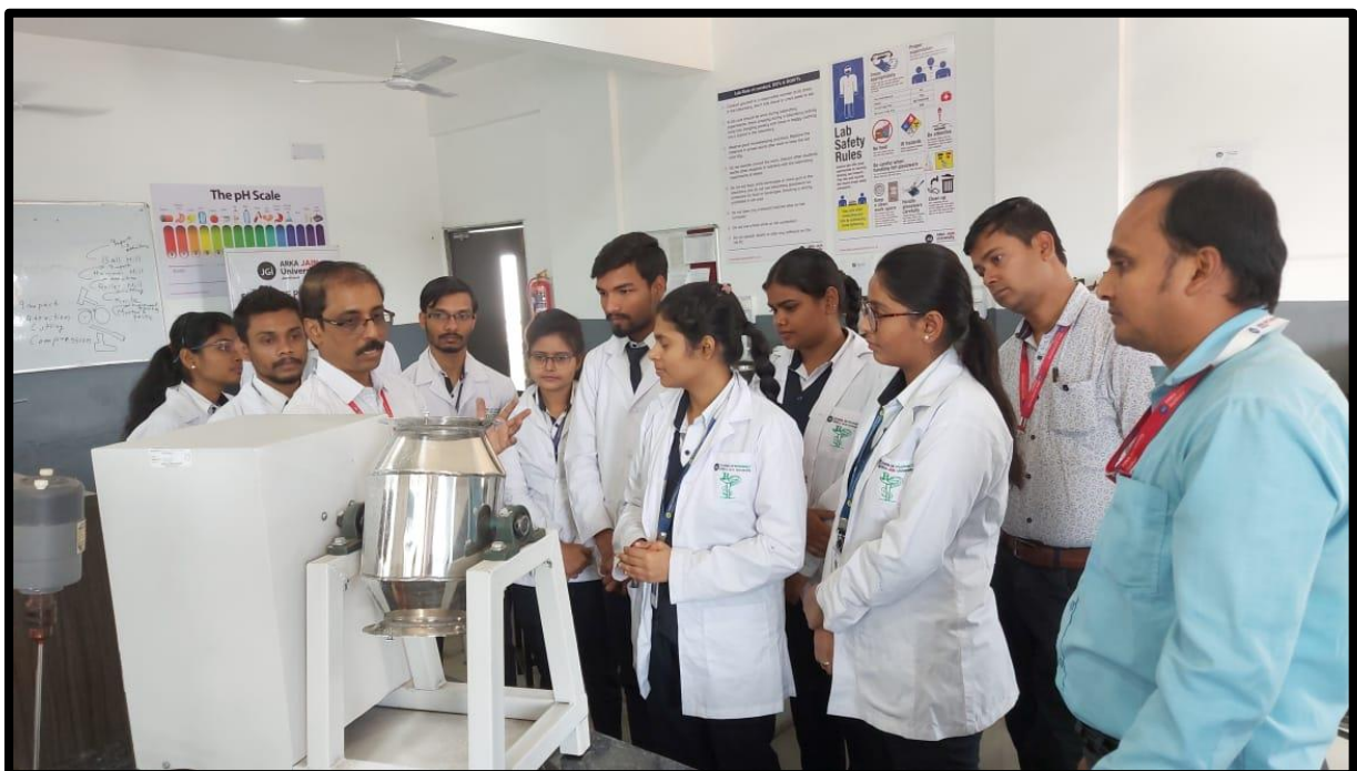
Figure 12: Instructor explaining the principle, construction and working of double cone blender “Theoretical and Practical Approach to Various Unit Operations in Pharmaceutical Engineering”
