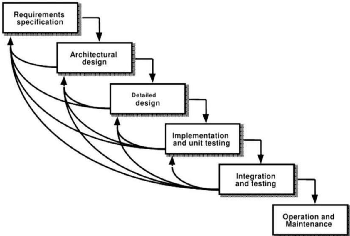
**Fig 1: Iterative Enhancement Model**
